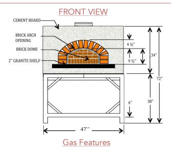
Gas connections ½ " NPT per burner, quick disconnect flex gas hose must be used. Pressure required 10" - 14" W.C. (Water Column) at the gas valve. 60,000 BTU's No electricity required
